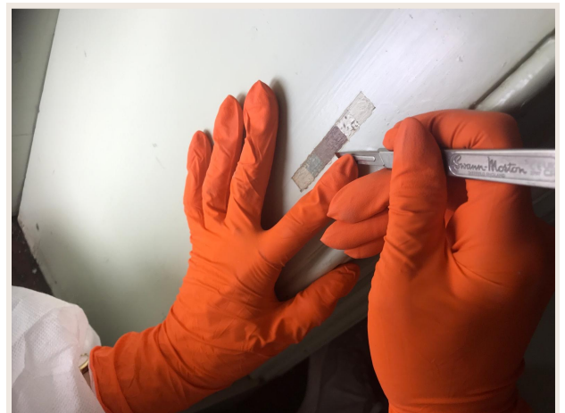
Fig. 4 The making of a stratigraphy on the north door with a scalpel knife. Photo by Dunya Verwey.
